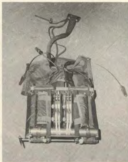
Left above, DART brake system on underside of seat. Right, stowage of snubber lines on each side of underside of seat.
